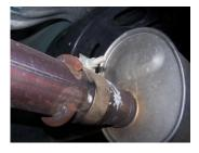
2. To remove your stock exhaust, remove the clamp located in front of the muffler. For easier removal, unbolt rear tailpipe hanger and grommet with a 13mm wrench. Then remove other hanger from rubber grommet, and cut off tailpipe just behind muffler. Now remove the rest of the system at the clamp.
