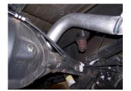
5. Slide tailpipe #C into muffler 1½"-2" and secure with clamp #F. Do not tighten. Insert welded hangers into rubber grommets.
