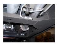
3. Install headpipe #A onto your existing stock flange and secure using the stock hardware. Do not tighten. Insert welded hanger into rubber grommet.
