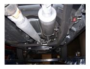
4. Install muffler #B onto headpipe 1½"-2" with the louvers facing towards the converter. Use a jack stand to support the muffler. Use clamp #F to secure the muffler to the headpipe. Do not tighten. Muffler inlet is looking into the louvers.
