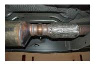
2. Remove the stock exhaust by unbolting it at the flange located in front of the muffler. Disengage the welded hangers from the OEM rubber grommets. Use WD-40 to aid in this process. Do not damage stock nuts and bolts or remove the rubber grommets as you will re-use them to mount your new system. Now, cut off tailpipe and remove system.
