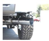
4. Next, slide exit pipe #B onto tailpipe. Use clamp #C to secure the exit pipe to the tailpipe. Do not tighten. Insert welded hangers into Rubber grommets
