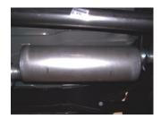
3. Install muffler #B onto head pipe #A 11/2"-2". Use a jack stand to support the muffler. Use clamp #E to secure the muffler to the headpipe. Do not tighten. Muffler outlet will be in the 11 o'clock position. Muffler inlet is looking into the louvers.
