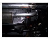
**3.** Install muffler #B onto head pipe #A  $1\frac{1}{2}$ "-2". Use a jack stand to support the muffler. DO NOT TIGHTEN. Muffler outlet is looking into the louvers.
