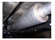
4. Install muffler #B onto head pipe 11/2"-2" with the louvers facing towards the converter. Use a jack stand to support the muffler. Use clamp #F to secure the muffler to the headpipe. DO NOT TIGHTEN. Muffler inlet is looking into louvers.
