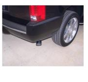
8. Install stainless steel tip. Clamp down. When you have everything in place, firmly tighten all bolts and clamps down securely. Use stainless steel cleaner and a Scotch Brite pad weekly to prevent tip from discoloration. Inspect all fasteners after 25-50 miles of operation and re-tighten as necessary.
