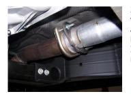
3. Install head pipe #A onto your existing stock flange and attach using the stock hardware. DO NOT TIGHTEN. Insert welded hanger into rubber grommet.
