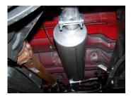
4. Install muffler #B onto headpipe #A 1.5-2" with louvers facing towards the converter. Use a jack stand to support the muffler. Outlet of muffler will be at 12 o'clock position.
