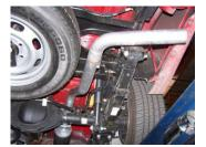
6. Install tailpipe #C into muffler 1.5-2". Insert welded hangers into rubber grommets. Use clamp #F to secure. Do not tighten.
