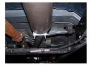
5. Next, install front muffler hanger #E onto muffler. Insert hanger into rubber grommets. Do not tighten.
