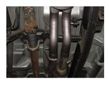
SLIDE PASSENGER SIDE HEADPIPE #A ONTO STOCK HEADPIPE. INSERT WELDED HANGER INTO RUBBER GROMMET. NEXT, INSTALL DRIVERS SIDE HEADPIPE #B ONTO STOCK HEADPIPE, USE CLAMP #H TO SECURE BOTH HEADPIPES, DO NOT TIGHTEN.
