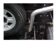
Install drivers side tailpipe # C into muffler 1-1/2" to 2". Rotate until it touches the rear mount, use clamp # H to secure tailpipe to muffler. Do not tighten.
