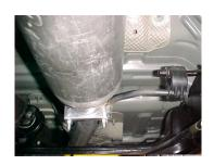
Next, install rear tailpipe hanger # G it will be installed just in front of the rear bed mount on the drivers side.
