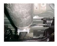
Next install front muffler hanger #E onto muffler. Insert hanger into rubber grommets. Do not tighten.
