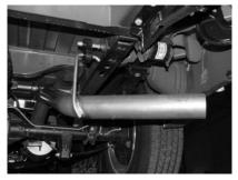
SLIDE OVERAXLE TAILPIPE #E INTO THE OUTLET OF THE MUFFLER 1 ½" TO 2". INSERT WELDED HANGER INTO RUBBER GROMMET AND CLAMP DOWN USING HANGER # D.
