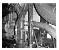
INSTALLTHE OVER AXLE TAILPIPE #C INTO THE OUTLET OF THE MUFFLER 1  $\frac{1}{2}$ " TO 2". DO NOT TIGHTEN. DO NOT TIGHTEN.
