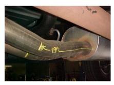
TO REMOVE STOCK EXHAUST, CUT 13" FROM THE FRONT OF THE MUFFLER.
