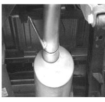
NEXT CONNECT THE MUFFLER TO THE HEADPIPE 1 ½" TO 2" USING CLAMP #E. TO SECURE MUFFLER TO PIPE, USE JACKSTANDS TO SUPPORT THE MUFFLER. THE OUTLET OF THE MUFFLER WILL BE AT APPROXIMATELY 11 O'CLOCK. THE MUFFLER INLET IS LOOKING INTO THE LOUVERS. DO NOT TIGHTEN.
