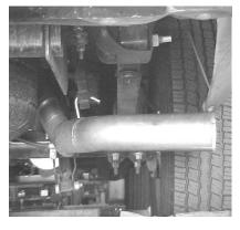
INSTALL EXIT PIPE #D ONTO OVERAXLE TAILPIPE USING CLAMP# E TO SECURE. ROTATE EXIT PIPE UNTIL IT IS AT THE CORRECT ANGLE FOR YOUR TRUCK. INSERT WELDED HANGER INTO RUBBER GROMMET.
