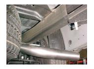
Install over axle tailpipe #C into muffler  $1\frac{1}{2}$ " to 2". Secure together with clamp #C. Do not tighten. Insert hanger into rubber arommet.
