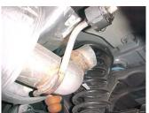
Lay out the exhaust on the floor so it looks like the drawing and compare parts with manual. To remove the stock exhaust remove it from the 2-bolt flange located behind the muffler cut your tailpipe off for easier removal. Leave all rubber grommets in place. Use WD-40 to aid in the removal of exhaust and hanger. Do not disgaurd stock hardware, you will reuse it.
