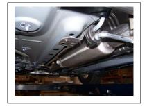
Install resonator # A on to your existing stock 2-bolt flange and secure with bolt kit # E. Use a jack stand to support the resonator.
