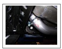
Install muffler # D onto the tailpipe.
