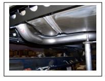
Install frontpipe # B 1-1/2" to 2" into the resonator. Use clamp # F to secure the tailpipe to the muffler. Do not tighten.
