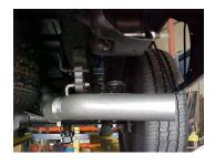
Install the turnout pipe #D on to the tailpipe. Secure together with clamp #F. Do not tighten. Roll the exit pipe until it is at the correct angle for your truck. Insert welded hanger into rubber grommet.
