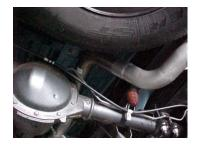
Insert welded hanger into rubber grommet.
