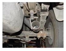
INSTALL EXIT PIPE #D ONTO THE TAILPIPE. ROTATE UNTIL IT IS LEVEL. USE CLAMP #F TO SECURE THE EXIT PIPE TO THE TAILPIPE. DO NOT TIGHTEN.
