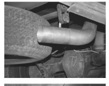
INSTALL TURNOUT #D PIPE ONTO TAILPIPE.
