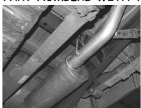
SLIDE OVERAXLE TAILPIPE #C INTO MUFFLER AT LEAST 1"-2". THE TAILPIPE END THAT GOES INTO THE OUTLET OF THE MUFFLER HAS THE LONGEST WELDED HANGER. SLIDE WELDED HANGERS INTO RUBBER GROMMETS. USE CLAMP # F TO SECURE PIPE TO MUFFLER. DO NOT TIGHTEN.
