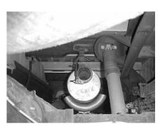
INSTALL MUFFLER ONTO HEADPIPES NO MORE THAN 1 ½" TO 2" USING CLAMPS #G. USE A JACKSTAND TO SUPPORT MUFFLER.
