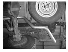
INSERT TURNOUT PIPE #E ONTO TAILPIPE AND ROTATE FOR YOUR DESIRED LOOK. USE CLAMP #H TO CONNECT TAILPIPE AND TURNOUT PIPE TOGETHER. DO NOT TIGHTEN.
