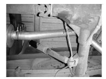
SLIP OVERAXLE PIPE #D INTO THE OUTLET OF THE MUFFLER NO MORE THEN 2" AND NO LESS THEN 1". SLIP WELDED HANGER INTO THE FACTORY RUBBER GROMMET AND ATTACH WITH CLAMP #H.
