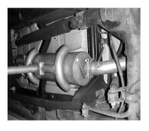
SLIDE MUFFLER WITH DUAL INLET ONTO HEADPIPE AT LEAST 1-1/2" TO 2".
