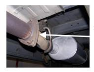
LAY OUT THE GIBSON EXHAUST ON THE FLOOR AND COMPARE PART #'S TO THE DRAWING. UNBOLT STOCK EXHAUST FROM BEHIND CATALYTIC CONVERTER. USE JACK STANDS TO SUPPORT CONVERTER SO IT WILL NOT DROP.
