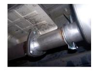
BOLT FRONT HEADPIPE #A ONTO STOCK FLANGE USING SUPPLIED BOLT KIT #H ANS GASKET #I. INSERT WELDED HANGER INTO RUBBER GROMMET.
