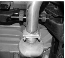
INSTALL REAR MUFFLER HANGER #E INTO RUBBER GROMMETS, LONGER SIDE OF THE HANGER WILL GO TOWARDS THE DRIVERS SIDE. THE CLAMP WILL BE USED TO SECURE THE TAILPIPE TO THE MUFFLER, DO NOT TIGHTEN.
