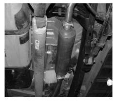
INSTALL MUFFLER #B ONTO HEADPIPE 1-1/2" TO 2" WITH INLET TOWARDS THE ENGINE. OUTLET SHOULD BE AT THE 12 O'CLOCK POSITION. USE CLAMP #F TO SECURE MUFFLER TO THE HEADPIPE, DO NOT TIGHTEN. THE INLET OF THE MUFFLER IS LOOKING INTO THE LOUVERS.
