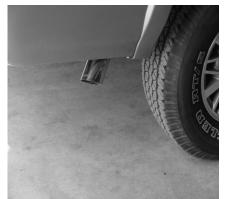
INSTALL YOUR STAINLESS TIP. TO CLEAN TIP USE ANY STAINLESS OR ALUMINUM CLEANER AND A SCOTCH BRITE PAD. NOW GO BACK AND TIGHTEN ALL CLAMPS, BOLTS AND NUTS.
