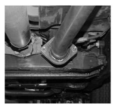
TO REMOVE STOCK EXHAUST **UN-BOLT IT FROM THE 2-BOLT** FLANGE LOCATED BETWEEN THE CATALYTIC CONVERTER AND THE MUFFLER. NOW CUT OFF YOUR STOCK TAILPIPE JUST BEHIND THE MUFFLER AND REMOVE. LEAVE ALL RUBBER GROMMETS ON THE HANGER. USE WD-40 TO AID IN REMOVAL OF EXHAUST AND HANGERS. INSTALL HEADPIPE #A, USE #G GASKET, NUTS AND BOLTS, KIT # H. INSERT WELDED HANGER INTO RUBBER GROMMET. DO NOT TIGHTEN.
