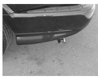
INSTALL THE OVERAXLE TAILPIPE #C INTO THE REAR OF THE MUFFLER AND ATTACH WITH CLAMP # G. BUT DO NOT TIGHTEN BEFORE INSTALLING EXIT PIPE. (REAR FACTORY TAILPIPE HANGER MUST BE UNBOLTED AND ROTATED 180 DEGREES) SEE PICTURE. THEN INSTALL EXIT PIPE #D ONTO OVERAXLE PIPE AND SLIDE WELDED HANGER ON PIPE INTO FACTORY REAR HANGER AND ATTACH WITH CLAMP # H.
