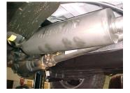
3. Slide muffler #A onto headpipe  $1\frac{1}{2}$ "-2". Use a jack stand to support the muffler. Make sure muffler outlets are level. Use clamp #G to secure the muffler to the headpipe. Do not tighten.
