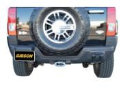
7. Install stainless steel tips. Clamp down. When you have everything in place, firmly tighten all bolts and clamps down securely. Use stainless steel or aluminum cleaner to polish tips. Inspect all fasteners after 25-50 miles of operation and re-tighten as necessary.
