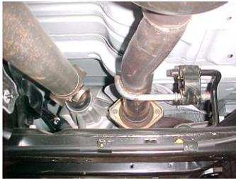
2. To remove the stock exhaust, unbolt it at the 2-bolt flange in front of the muffler. Disengage the welded hangers using WD-40 from the OEM rubber grommets. Do not damage or remove the rubber grommets as you will re-use them to mount your new system.
