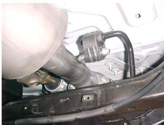
3. Install headpipe #A onto your existing stock flange using bolt kit #H to secure flange. DO NOT TIGHTEN. Insert welded hanger into rubber grommet.
