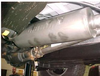
4. Install muffler #B onto headpipe 1 1/2"-2". Use a jack stand to support the muffler. Make sure muffler outlets are level. Use clamp #G to secure the muffler to the headpipe. DO NOT TIGHTEN.
