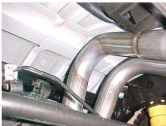
5. Slide driver side over axle tailpipe #C into muffler 1.5-2". Use clamp #G to secure tailpipe to muffler. Do not tighten. Insert welded hanger into rubber grommet.
