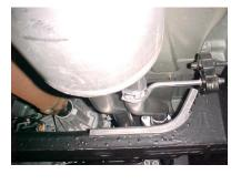
Install muffler #C onto head pipes 1-1/2" to 2" with the louvers facing towards the converter. Use a jack stand to support the muffler. Use clamps #G to secure the muffler to the head pipes. Do not tighten. Outlet of muffler should be at 6 o'clock.
