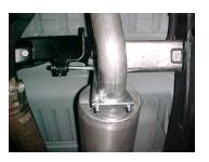
Install rear muffler hanger #F onto outlet of muffler. And clamp down to tailpipe. Insert hanger into rubber grommet. Do not tighten.
