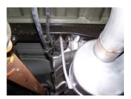
7. Install band clamp #F onto muffler. Insert hanger into rubber grommet. Use provided bolt kit #H. Do not tighten.
