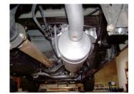
6. Slide muffler #C onto the resonator 1.5-2". Use clamp #G to secure muffler to resonator. Do not tighten. Outlet will be at the 12 o'clock position. Inlet of muffler will be looking into the louvers.
