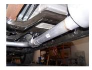
5. Slide resonator #B onto the Y Pipe 1½"-2". Use clamp #G to secure pipes together. Do not tighten.
