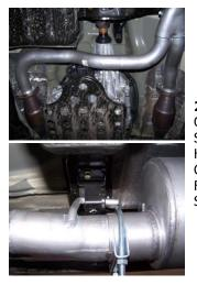
2. INSTALL Y-PIPE # A ONTO YOUR EXISTING STOCK FLANGES. INSERT HANGER INTO RUBBER GROMMET. USE YOUR FACTORY HARDWARE TO SECURE. DO NOT TIGHTEN.
