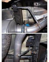
**4.** INSTALL OVERAXLE TAILPIPE # C INTO MUFFLER 1½"-2". INSERT WELDED HANGERS INTO RUBBER GROMMETS. SECURE TO THE MUFFLER USING CLAMP # E. DO NOT TIGHTEN.
