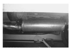
INSTALL MUFFLER # B ONTO HEAD PIPE # A 1-1/2" TO 2" WITH THE LOUVERS FACING TOWARDS THE CONVERTER. USE A JACK STAND TO SUPPORT THE MUFFLER. USE CLAMP # E. TO SECURE THE MUFFLER TO THE HEAD PIPE. DO NOT TIGHTEN. MUFFLER INLET IS LOOKING INTO THE LOUVERS. OUTLET OF MUFFLER WILL BE AT THE 1 O'CLOCK POSTION.
