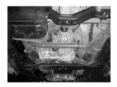
LAY OUT THE GIBSON EXHAUST ON THE FLOOR AND COMPARE PART #'S TO THE DRAWING. TO REMOVE THE STOCK EXHAUST REMOVE IT FROM THE 2 BOLT FLANGES, LOCATED IN FRONT OF YOUR FACTORY MUFFLER. NEXT, CUT IFF YOUR STOCK TAILPIPE BEHIND YOUR MUFFLER. DO NOT DISGARD YOUR FACTORY HARDWARE, YOU WILL RE-USE IT.
