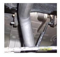
**INSTALL HEADPIPE #A** ONTO STOCK PIPE, USE CLAMP# E TO SECURE PIPES TOGETHER. DO NOT TIGHTEN. NEXT, MOUNT WELDED HANGER TO RUBBER GROMMET USING BOLT KIT # F.
