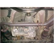
LAY OUT THE GIBSON EXHAUST ON THE FLOOR AND COMPARE PART #'S TO THE DRAWING. TO REMOVE YOUR FACTORY EXHAUST UN-BOLT YOUR TAILPIPE AT THE 2-BOLT FLANGE LOCATED BEHIND YOUR STOCK MUFFLER USE WD-40 TO AID YOU IN REMOVAL OF HANGERS FROM RUBBER GROMMETS. DO NOT DAMAGE THE GROMMETS,
