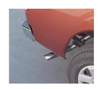
INSTALL YOUR STAINLESS TIP TO YOUR DESIRED LOOK. NOW GO BACK AND TIGHTEN ALL YOUR FLANGES, CLAMPS, ETC. STARTING FROM THE FRONT AND WORKING YOUR WAY BACK. TO CLEAN YOUR STAINLESS TIP USE A STAINLESS CLEANER AND A SCOTCH BRITE PAD. AFTER 20-25 MILES CHECK AND RETIGHTEN ALL FASTENERS IN NESERSARY.
