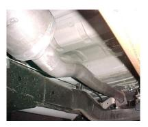
SLIDE HEADPIPE # A ONTO YOUR FACTORY PIPE 1-1/2" TO 2". USE CLAMP # F TO SECURE. DO NOT TIGHTEN.
