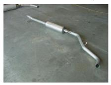
LAY OUT THE GIBSON EXHAUST ON THE FLOOR AND COMPARE PART NUMBERS WITH THE MANUAL. LEAVE ALL FACTORY GROMMETS IN PLACE. FOR EASIER REMOVAL OF GROMMETS AND HANGERS USE WD-40 ON THEM.
