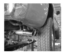
INSTALL THE STAINLESS TIPS. NOW GO BACK AND START AT THE FRONT AND TIGHTEN ALL CLAMPS AND HANGERS.
