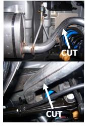
2. To remove the stock exhaust, Un clamp it from the clamp in front of the muffler. Do not disguard you will re-use clamp. Disengage the welded hangers using WD-40 from the OEM rubber grommets. Do not damage or remove the rubber grommets as you will reuse them to mount your new system. Now, cut off tailpipe before and after rear axle for removal.
