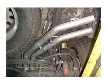
ATTACH BOTH TAILPI PES USING BOLT KIT # I. THE PASSENGER SIDE MOUNTING BRACKET WILL BE POSITIONED UNDERNEATH THE DRIVERSIDE. NOW GO BACK AND TIGHTEN ALL CLAMPS, HANGERS AND BOLTS.
