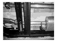
LAY OUT THE GIBSON EXHAUST ON THE FLOOR AND COMPARE PART #'S TO THE DRAWING. TO REMOVE STOCK EXHAUST, REMOVE IT FROM THE 2-BOLT FLANGE LOCATED IN FRONT OF THE MUFFLER. DO NOT DISGUARD FACTORY HARDWARE YOU WILL RE-USE IT. LEAVE ALL RUBBER GROMMETS IN PLACE. USE WD-40 TO AID IN REMOVAL OF EXHAUST AND THE RUBBER GROMMETS.
