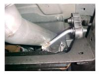
INSTALL HEAD PIPE # A ONTO YOUR EXISTING STOCK FRONT PIPE. INSERT WELDED HANGER INTO RUBBER GROMMET. YOU WILL BE USING THE FACTORY HARDWARE.
