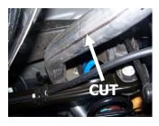
**3. 2009-10 Models Only** Measure 8" from the flange on your new headpipe #A and cut. Attach adapter pipe to new headpipe with the 3" clamp. You will re-use the factory band clamp.
