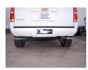
**7.** Install driver side tailpipe #C into the muffler 1½-2". Use clamp #G to secure tailpipe to muffler. DO NOT TIGHTEN. Insert welded hangers into rubber grommets.
