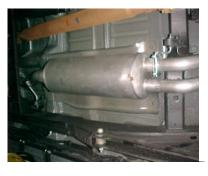
INSTALL MUFFLER # B ONTO HEAD PIPE 1-1/2"-2" WITH THE LOUVERS FACING TOWARDS THE CONVERTER. USE A JACK STAND TO SUPPORT THE MUFFLER. USE CLAMP # F TO SECURE THE MUFFLER TO THE HEADPIPE. DO NOT TIGHTEN.
