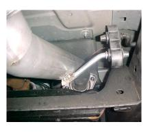
BOLT HEADPIPE # A ONTO YOUR EXISTING STOCK FRONT PIPE RE-USING FACTORY BOLTS. INSERT WELDED HANGER INTO RUBBER GROMMET.
