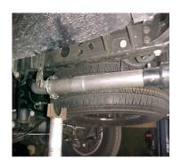
NEXT, INSTALL THE EXIT PIPES #E AND #F USEING CLAMPS #H TO SECURE TO THE TAILPIPES. DO NOT TIGHTEN.
