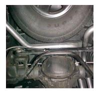
INSTALL THE PASSENGER SIDE OVERAXLE TAILPIPE #D TO THE MUFFLER 1-1/2"-2". USE CLAMP # H TO SECURE TAILPIPE TO MUFFLER. DO NOT TIGHTEN.
