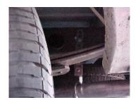
Install metal hangers # I Into holes located approximately 22" from the rear of the frame. Metal hangers are mounted on the outside of the frame. Use the hardware that is provided. The bolt and the washer will go into the 3<sup>rd</sup> hole from the top of the hanger. You may need to loosen spare tire for easier installation.
