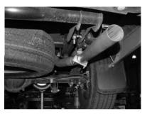
INSTALL PASSENGER SIDE TAILPIPE #C INTO MUFFLER AT LEAST 1 1 TO 2". USE CLAMP #G TO SECURE PIPE TO MUFFLER. DO NOT TIGHTEN. THE TAILPIPES WILL BOTH LEAN TOWARDS THE DRIVER SIDE FOR CLEARANCE.
