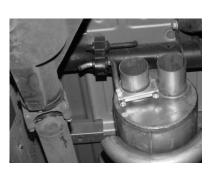
INSTALL MUFFLER #B ONTO HEADPIPE AT LEAST 1 1/2" TO 2". USE CLAMP #F TO SECURE MUFFLER TO HEADPIPE. DO NOT TIGHTEN. USE A JACK STAND TO SUPPORT THE MUFFLER. OUTLETS SHOULD BE AT THE TOP.
