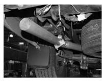
INSTALL DRIVER SIDE TAILPIPE #D INTO MUFFLER AT LEAST 1 1/2" TO 2". THIS PIPE WILL ROUTE OVER THE AXLE AND BETWEEN THE SHOCK AND SPARE TIRE. USE CLAMP #G TO SECURE PIPE TO MUFFLER, DO NOT TIGHTEN. INSERT WELDED HANGER INTO RUBBER GROMMET.
