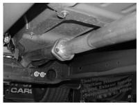
**BOLT HEADPIPE #A TO STOCK** FLANGE RE-USING FACTORY WELDED HANGER INTO RUBBER
