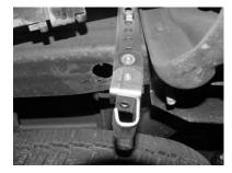
INSTALL METAL HANGERS #H INTO HOLES LOCATED APPROX. 16" FROM THE REAR OF THE FRAME. METAL HANGERS ARE MOUNTED ON THE OUTSIDE OF FRAME. USE HARDWARE KIT # I. THE BOLT AND WASHER WILL GO INTO THE 3RD HOLE FROM THE TOP OF THE HANGER.
