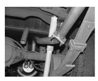
INSTALL PASSENGER SIDE TAILPIPE # C INTO THE MUFFLER 1-1/2" TO 2". ATTACH IT TO THE MUFFLER USING CLAMP # I. THEN USE CLAMP # I TO HOLD TAILPIPE TO HANGER # F. DO NOT TIGHTEN
