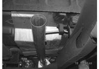
UNBOLT STOCK HEADPIPE AT THE 3 BOLT FLANGE DIRECTLY BEHINDTHE CATALYTIC CONVERTER. CUT STOCK TAILPIPE OFF RIGHT BEHIND THE STOCK MUFFLER. LEAVE ALL FACTORY RUBBER GROMMETS IN PLACE. SPRAY WD-40 ON ALL RUBBER GROMMETS FOR EASY REMOVAL.
