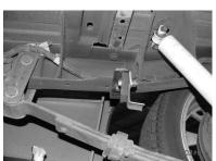
INSTALL HANGER # F ON THE PASSENGER TAILPIPE AND HANGER # G ON DRIVERSIDE TAILPIPE. MEASURE 19" FROM REAR OF FRAME AND BOLT INTO THE EXISTING ROUND HOLES (ABOUT 7/8") LOCATED ON THE FRAME ON BOTH SIDES OF THE VEHICLE
