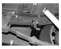
INSTALL HANGER # F ON THE PASSENGER TAILPIPE AND HANGER # G ON DRIVERSIDE TAILPIPE. MEASURE 19" FROM REAR OF FRAME AND BOLT INTO THE EXISTING ROUND HOLES (ABOUT 7/8") LOCATED ON THE FRAME ON BOTH SIDES
