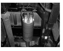
INSTALL MUFFLER #B ONTO HEADPIPE 1-1/2" TO 2" USING CLAMP #J. INSERT WELDED HANGERS INTO RUBBER GROMMET. MAKE SURE OUTLETS ARE LEVEL. USE A JACKSTAND TO SUPPORT MUFFLER.
