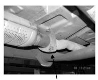
UNBOLT STOCK HEADPIPE AT THE 2- BOLT FLANGE DIRECTLY BEHIND THE CATALYTIC CONVERTER. CUT STOCK TAILPIPE OFF RIGHT BEHIND THE STOCK MUFFLER. LEAVE ALL FACTORY RUBBER GROMMETS IN PLACE. SPRAY WD-40 ON ALL RUBBER GROMMETS FOR EASY REMOVAL.
