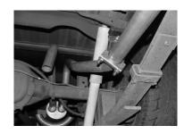
INSTALL PASSENGER SIDE TAILPIPE # C INTO THE MUFFLER 1-1/2" TO 2". ATTACH IT TO THE MUFFLER USING CLAMP # I. INSERT WELDED HANGER INTO RUBBER GROMMET AND USE CLAMP # I TO HOLD TAILPIPE TO HANGER # F. DO NOT TIGHTEN
