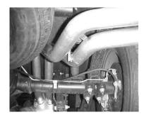
USING CLAMP #G & HANGER # H CONNECT BOTH TAILPIPES TO THE OUTLETS OF THE MUFFLER. ROTATE TAILPIPES TO BEST FIT YOUR TRUCK.
