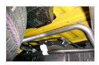
7. Install driver side tailpipe (**#C**) into muffler 1.5-2". Rotate until it touches the rear mount, use clamp (**#H**) to secure tailpipe to muffler. Do not tighten.
