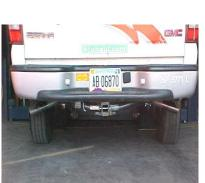
INSTALL THE PASSENGER SIDE TAILPIPE #C INTO MUFFLER AT LEAST 1 ½" TO 2". USE CLAMP (#G) TO SECURE PIPE TO MUFFLER. DO NOT TIGHTEN. THE TAILPIPES WILL BOTH LEAN TOWARDS THE DRIVER SIDE LOOKING FROM THE REAR OF THE VEHICLE - THIS TAILPIPE IS AT APPX. 11 O'CLOCK.
