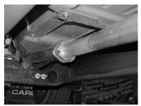
BOLT HEADPIPE (#A) TO STOCK FLANGE RE-USING FACTORY NUTS. DO NOT TIGHTEN. SLIDE WELDED HANGER INTO RUBBER GROMMET
