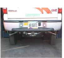
INSTALL PASSENGER SIDE TAILPIPE (#C) INTO MUFFLER AT LEAST 1  $\frac{1}{2}$ " TO 2". USE CLAMP #G TO SECURE PIPE TO MUFFLER. DO NOT TIGHTEN. THE TAILPIPES WILL BOTH LEAN TOWARDS THE DRIVER SIDE LOOKING FROM THE REAR OF THE VEHICLE.
