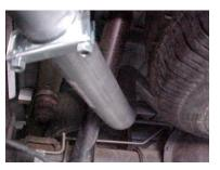
INSTALL DRIVER SIDE TAILPIPE (#D) INTO MUFFLER AT LEAST 1 ½" TO 2". THIS PIPE WILL ROUTE OVER THE AXLE, BETWEEN THE SHOCK AND SPARE TIRE. ATTACH CLAMP #9 TO SECURE TAILPIPE TO MUFFLER. DO NOT TIGHTEN. LOOKING FROM INSERT WELDED HANDER INTO RUBBER GROMMET.
