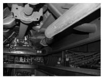
TO REMOVE STOCK EXHAUST UNBOLT IT FROM THE FLANGE LOCATED JUST BEHIND THE FACTORY Y-PIPE. YOU WILL RE-USE YOUR FACTORY BOLTS FROM FLANGE. NOW, CUT OFF YOUR STOCK TAILPIPE JUST BEHIND THE MUFFLER AND REMOVE. LEAVE ALL RUBBER GROMMETS ON THE HANGER. USE WD-40 TO AID IN REMOVAL OF THE EXHAUST AND HANGERS.
