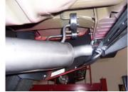
4. Install driver side muffler assembly #A. Insert welded hangers into rubber grommets. Use clamp #D to secure pipes together. Do not tighten.
